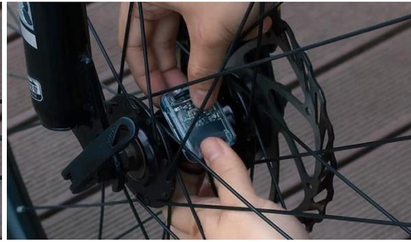
3. With the rubber holder in contact with the wheel hub, attach the rubber ring on the opposite side to affix it.
