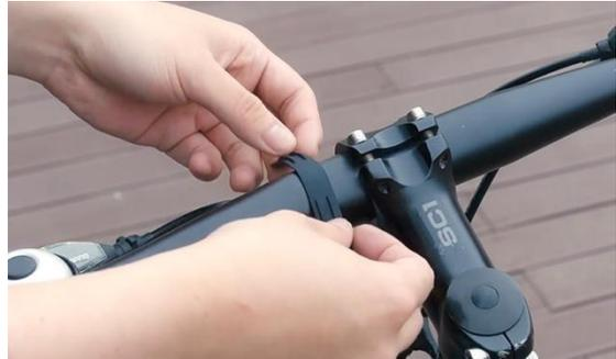
3. After fitting the mount to the groove of the rubber band, use a 2.5mm screw and a hexagon wrench to tighten the
